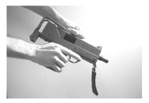
② While holding cocking knob, pull trigger and ease bolt forward into closed position.
