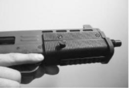
(3) Hold upper and lower receiver together with one hand and with other hand grasp protruding head of retaining pin and pull out.
