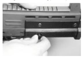
4 Slide grip forward and away from upper receiver. Do not pivot grip downward when removing or you may risk breaking the front of the grip.
