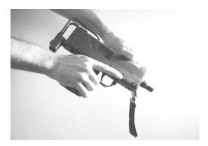
(3) Remove front pushpin and detach upper receiver from lower receiver.
