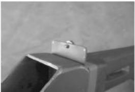
(5) With front grip and retaining pin removed from MAX-10/45 Slowfire Upper Receiver, slide rear of upper receiver assembly into rear of lower receiver until receiver holes align.
