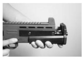
(5) Remove upper receiver from lower receiver.
