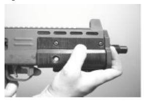
8 Push retaining pin through right side until fully seated.
